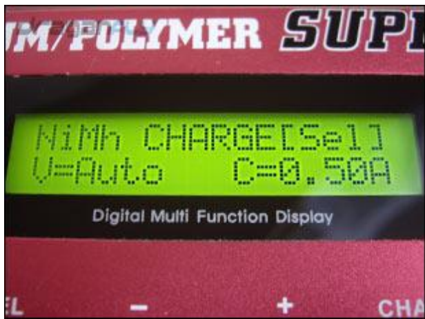
The Thunder Power 1010C with V2.3a Can Charge your NiMh Battery Packs
